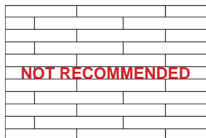
Brick bond installation 50% (NOT RECOMMENDABLE)
